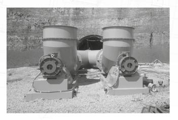
As a result, ZVVZ mine fans meet all the demanding requirements for reliable mine ventilation and gas mines and have all the necessary certificates. In this respect, our axial fans are unsurpassed in their reliability due to their simplicity of design, low maintenance and, above all, the fact that the principle of operation of the fan impeller makes it easy to ensure that it is explosion-proof.
