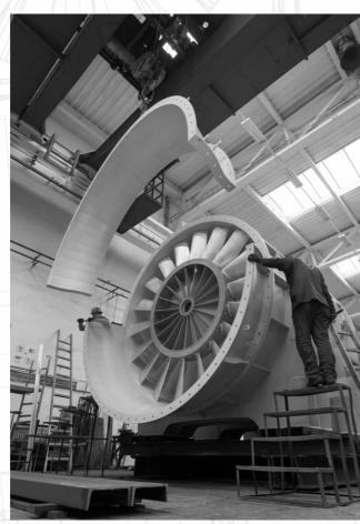
The fans for wind tunnels are supplied by ZVVZ with all turnkey accessories, i.e. including the drive and its cooling, modern service software, etc.
