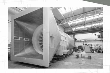
Therefore, the ZVVZ cooperates with leading research institutes both in the field of state-of-the-art composite materials for the production of impeller blades, and in the field of aerodynamics and acoustics. Thanks to this, the ZVVZ fans for wind tunnels work with very high efficiency. Efficiency above 90% is no longer any exception nowadays, and it rather belongs within standards of the machine. In addition, these fans are designed
