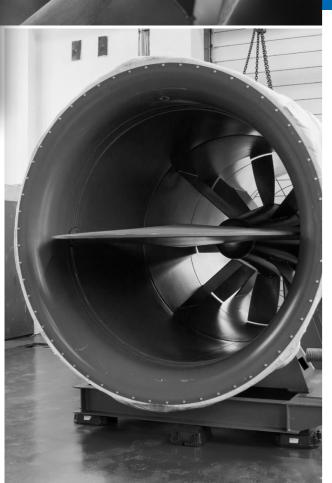
THE FANS ARE DESIGNED FOR THE DIAGONAL VENTILATION OF ROAD AND RAILWAY TUNNELS AND METRO TUNNELS DURING VENTING AND EMERGENCY VENTILATION.
