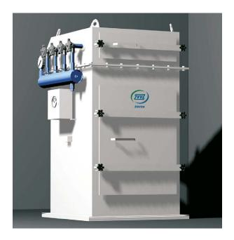
These are intended for separating solid particles from the flow of gas when ventilating silos and when extracting small volumes of gas of a volume of up to 9 000 m $^3$ /h and a temperature of up to 140 °C. The hoses are installed and replaced from the working side of the filter through a side door, which is also used to inspect the hoses. EFV bag filters are supplied to the construction site assembled, including the control unit, in several versions.
