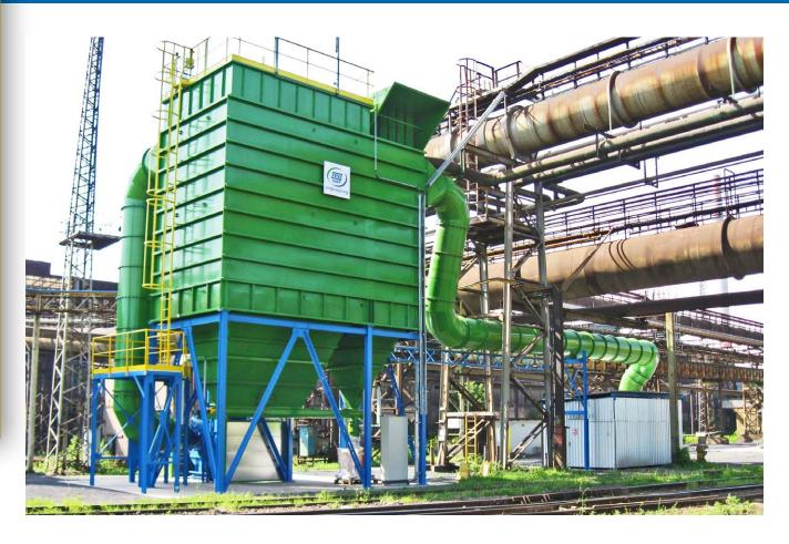
On-line bag EFP filters are mostly used in cement works, lime kilns or in quarries. They are designed for high input concentrations and have a specially designed polluted gas inlet for this purpose.
