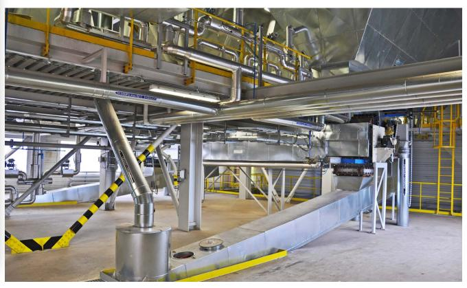
Pneumatic chute transport is suitable for high transport throughput rates (up to 400 t/h) over shorter distances, where room for the necessary slope is available. A transport chute is a modular structure, which enables various transport line setup designs: material input from several places, branches, Y-branches and material outfall, including inspection openings, transport air inlet and bleeding.
